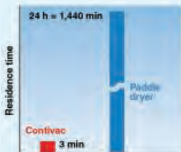
FIGURE 2. In this test, product was tested in both an h-PTFD and a batch paddle dryer. The difference was almost a factor of 500
