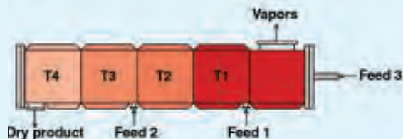
FIGURE 4. By splitting the heating jacket into different heating zones and placing multiple feed nozzles along the axis of the dryer, an h-PTFD can maximize process control flexibility
