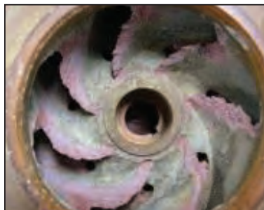
FIGURE 2. The degree of pump wear is expressed as the percent reduction in total head
