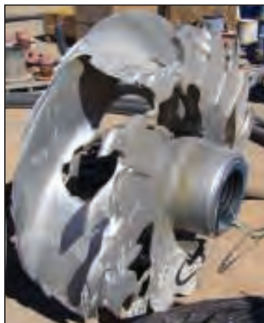
FIGURE 1. Pump wear, such as that shown on this pump impeller, can lead to reduced pump performance
