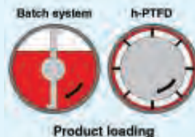
FIGURE 1. Product hold-up in a batch paddle dryer (left) is much larger than that achieved in an h-PTFD
